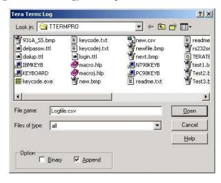
6. Press the PRINT button and one record of comma separated data should appear in the Tera Term Pro terminal window and simultaneously be recorded in the Tera Term:log file.
