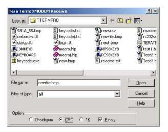
6. Press Enter, or click the Open button and a XMODEM Receive window should appear that shows bytes received. None should be received yet.
