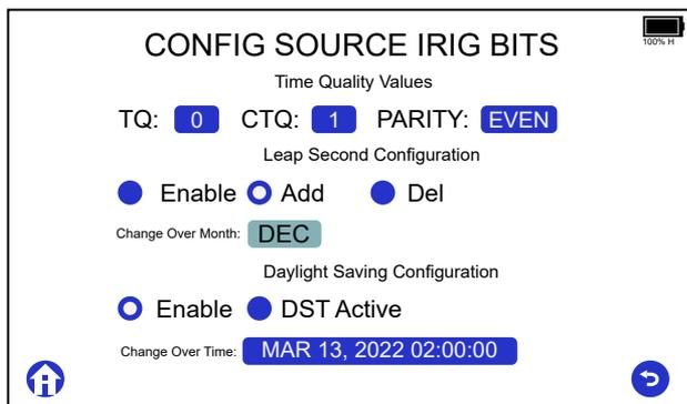
Figure 8: IRIG-B Source Bits Configuration Screen
