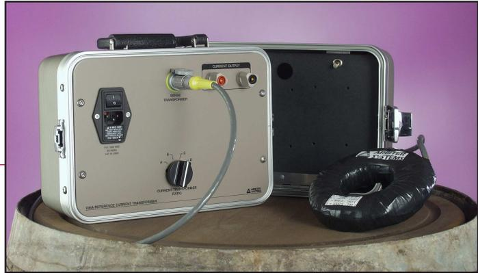
The Arbiter Systems<sup>®</sup>, Inc. Model 936A Reference Current Transformer provides laboratory grade accuracy in a small, portable, ruggedized case, making it ideal for field use. Multiple ratios of 1200:5, 1000:5, 800:5, 600:5 are selectable via a front panel switch. The guaranteed accuracy over the full input range and operating conditions is 0.02% ratio and 0.01° phase (traceable to NIST), ideal for calibrating other current transformers.
