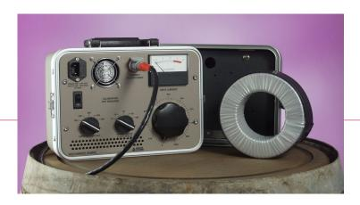
The Arbiter Systems®, Inc. Model 935A is designed to drive high currents, up to 1000 amps rms, through low impedance loads. Output current is produced at the input line frequency through a toroidal current transformer. The input line level is selectable from 100 Vrms, 120 Vrms, 200 Vrms, 220 Vrms, and 240 Vrms. An output range selector switch and variable transformer allow easy setting of the output current within the attainable range.
