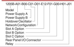
Redundant GNSS receiver
