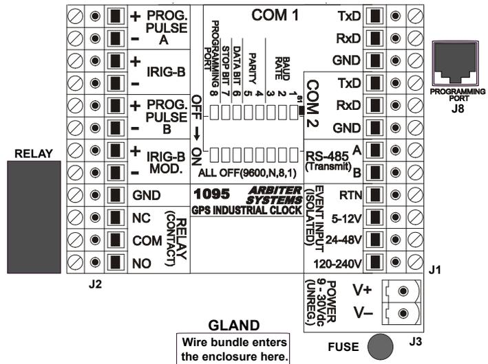
See *Main Gland Specifications* in the operation manual for details about wire type, especially if the clock is mounted outside. NOTE: Strip the wire insulation about 1/4 in and DO NOT TIN the bare wire with solder.
