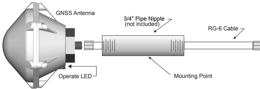
1. Pass the antenna cable through the pipe nipple and attach the cable to the antenna. Tighten by hand, and do not spin the antenna onto the cable connector, as it may damage the antenna/cable connection.
