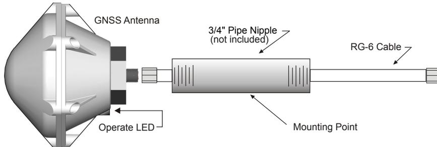
1. Pass the antenna cable through the pipe nipple and attach the cable to the antenna. Tighten by hand, and do not spin the antenna onto the cable connector, as it may damage the antenna/cable connection.
