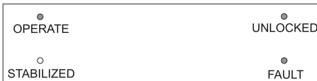
Figure 4.3: Model 1095A with Startup Fault
