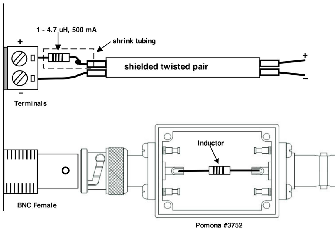
Figure 1: Connecting an Inductor to Output with Terminals & BNC Connector
