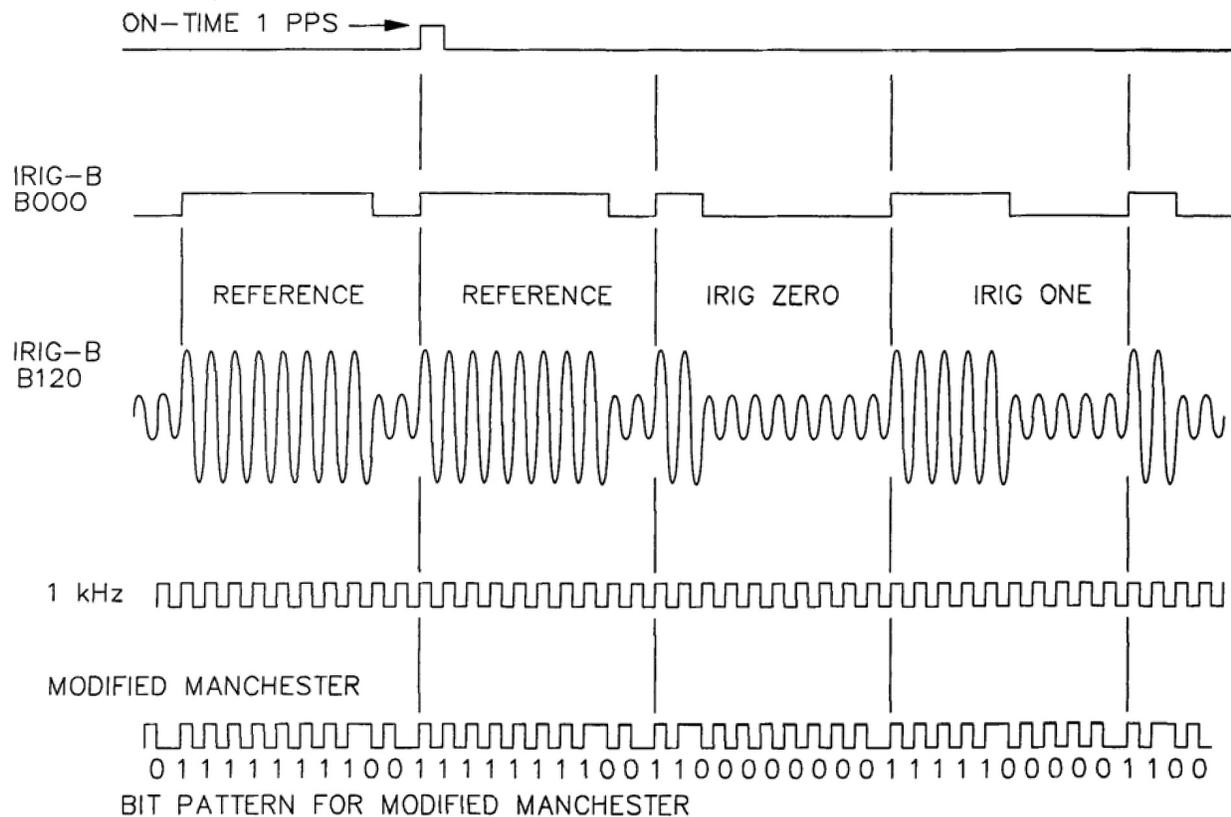
IRIG-B coding comparisons: level shift, 1 kHz amplitude modulated, and Modified Manchester.
